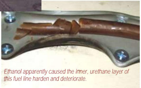
*Ethanol apparently caused the inner, urethane layer of this fuel line harden and deteriorate.*
