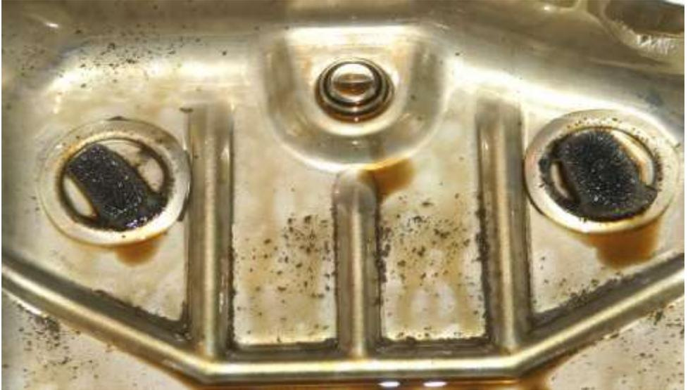
Magnets showing amount of debris attached
